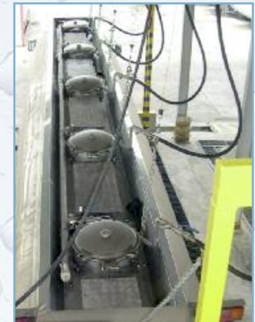
Simultaneous cleaning of several compartments of a road tanker.
