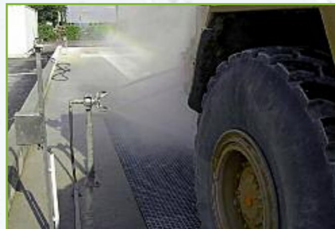
Chassis and frame washing.
