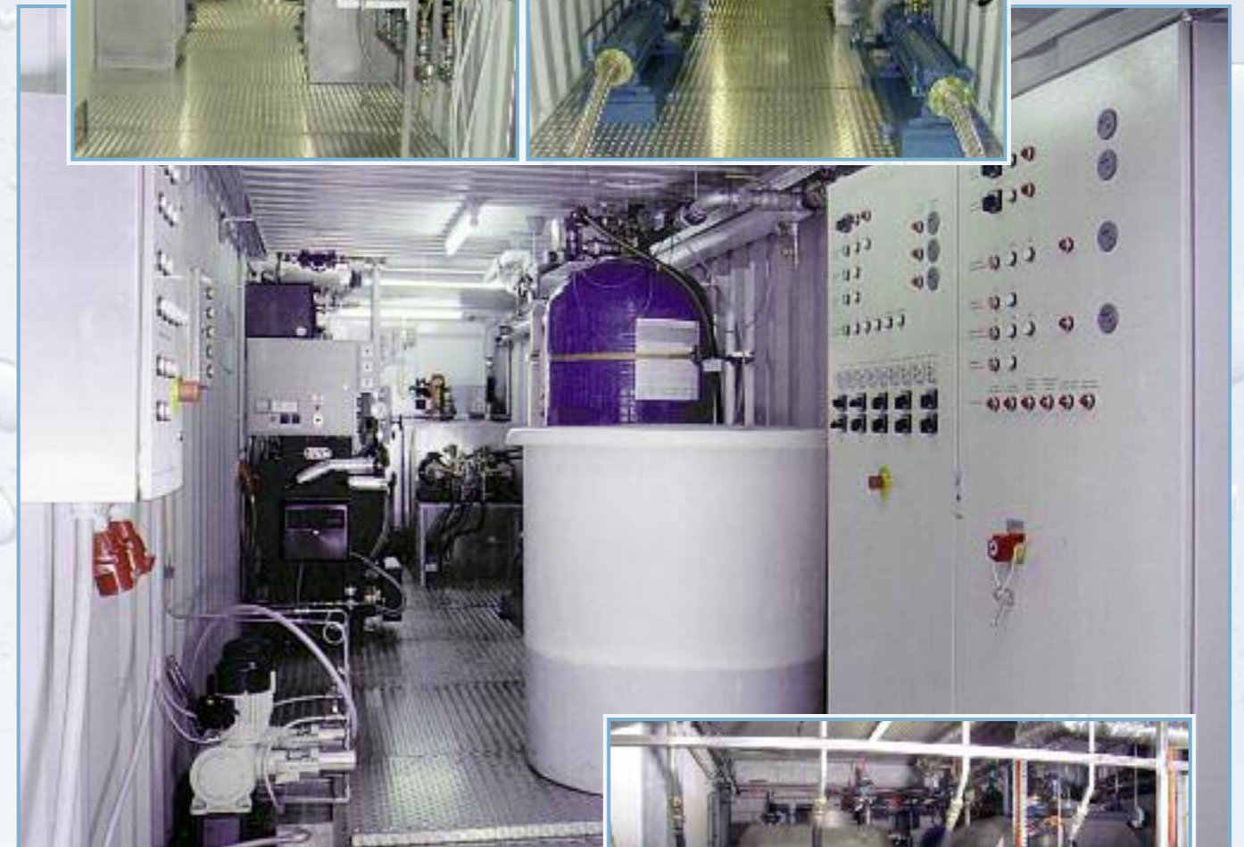
Cleaning technology built into a 40' container box.
