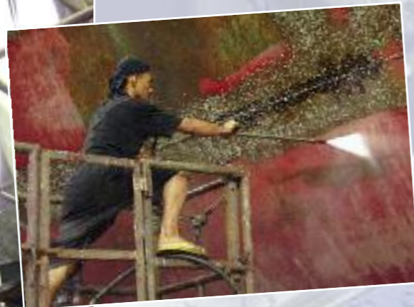
Application of a 400 bar high pressure cleaner in a chinese dry-dock.
