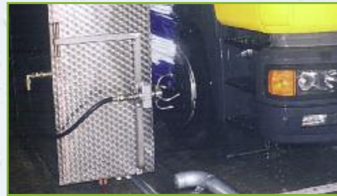
Chassis and wheel wash system connected to a truck washing machine.
